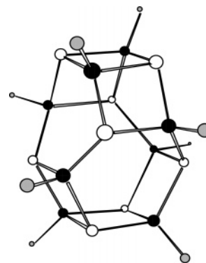
Figure 19. N 8 C 8 H 8 cage isomer in which all framework bonds are C–N bonds (symmetry point group S 4 ). This isomer has more C–N bonds than the other isomers in this study but suffers from ring strain in the additional four-membered rings.
